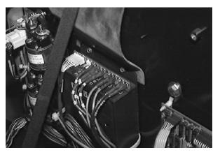
7. Disconnect, remove, and set aside the on/off key switch, hourmeter, and circuit breakers from the right hand side of the shroud. (Refer to FIG. 1)
